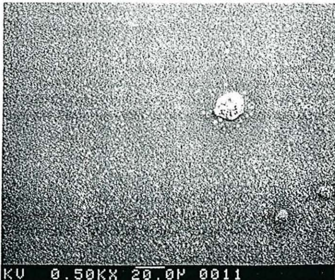
Fig. 4. SEM image at higher magnification of the line of Fig. 3. Notice that the film is uniform and crack-free.
