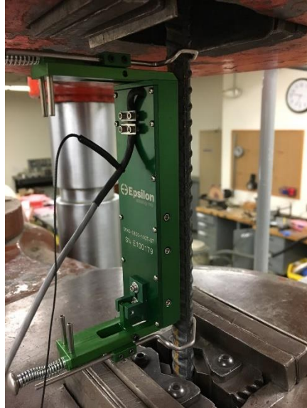
Figure 3 - 4: Tensile testing of reinforcing steel. The digital extensometer (Green) is attached to the rebar via clips. Rebar is loaded into UTM. (Image courtesy of Ian Williams).
