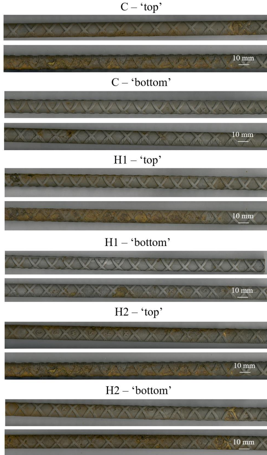
Figure 3 - 13: Representative scans of corrosion damage to reinforcing steel following excavation. The first image in each pair shows the side of the rebar closest to side A, while the second image shows the side closest to side C.
