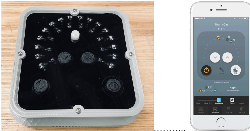
Figure 33: Prototype wall unit with underlying Hamilton and mobile phone interface.
