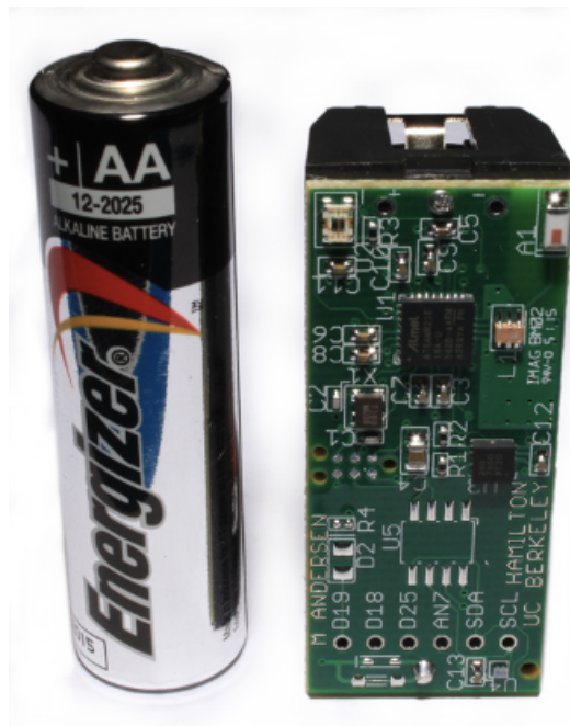
Figure 3: Photo of Hamilton 7 with typical AA battery, at cost of $9.80.
