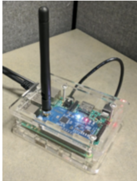
Figure 7: The border router based on a Raspberry Pi 3 miniature computer plus Hamilton-derived 802.15.4 interface in robust enclosure.
