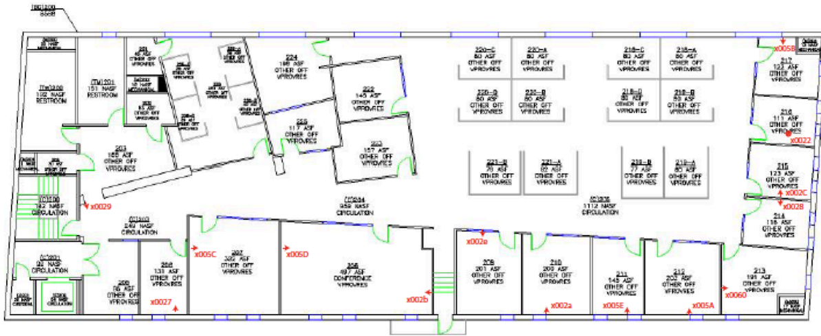
Figure 42: Floor plan of the CIEE offices in downtown Berkeley with location of Hamilton sensors in red.
