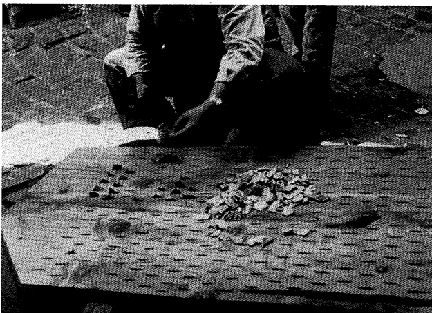
Figure 22.9 Sledge maker inserting flints in slots of sledge underbody, city of Urfa
