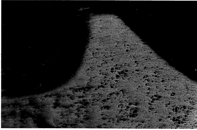
Figure 25.11 Predominantly parallel orientation of the striations on the tool in figure 25.10
