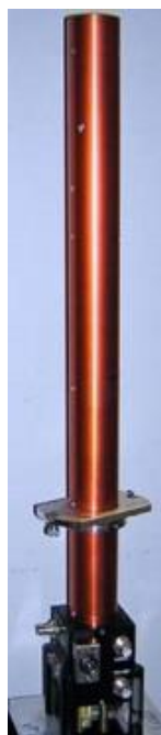
Figure A.1. A Varian ASWPFG broadband NMR probe. Two channels with two nuclei per channel are available on this probe, making it a 4-nucleus probe. This image shows the probe as it would appear when removed from the NMR.
