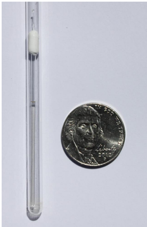
Figure A.6. Showing the capillary tube in the NMR tube. Enough deuterated solvent should be added to fill the NMR tube to about the same level as the level of the electrolyte in the capillary.
