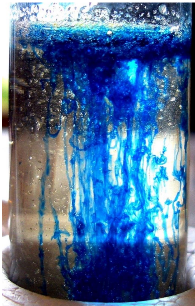
Figure 4.1. Aqueous precipitation of Prussian blue. Used with permission under the creative commons license from: https://www.flickr.com/photos/jurvetson/6627153/
