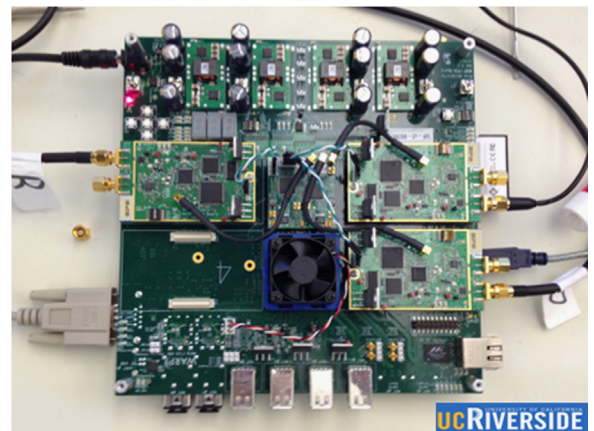
Fig. 1. A programmable radio board (WARP) where the TDTB method with n_r=1 and n_t=2 was tested. The FPGA on radio board was reprogrammed to accommodate the time domain approach.
