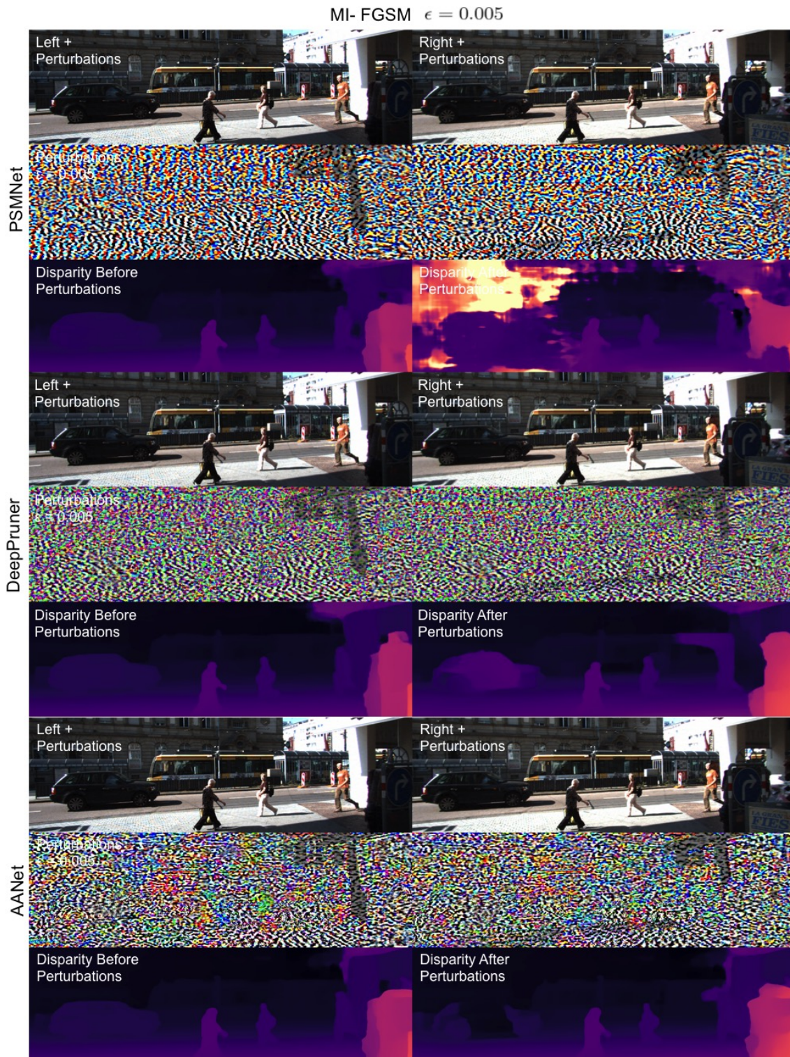
Figure A.5: Examples of MI-FGSM attacks using \epsilon = 0.005 .
