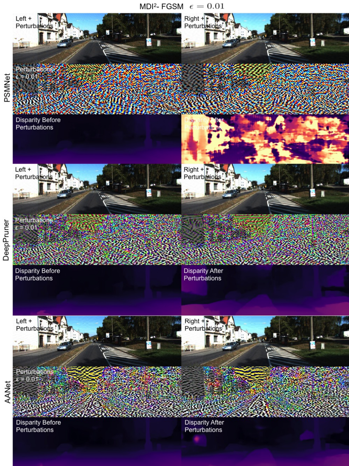
Figure A.10: Examples of MDI 2 -FGSM attacks using \epsilon = 0.01 .
