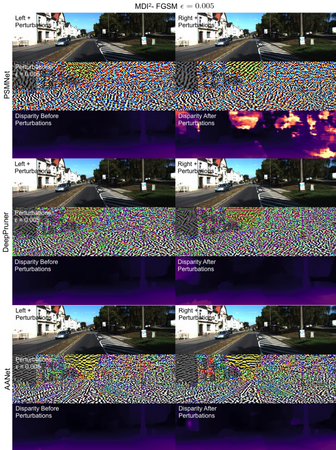
Figure A.9: Examples of MDI 2 -FGSM attacks using \epsilon = 0.005 .
