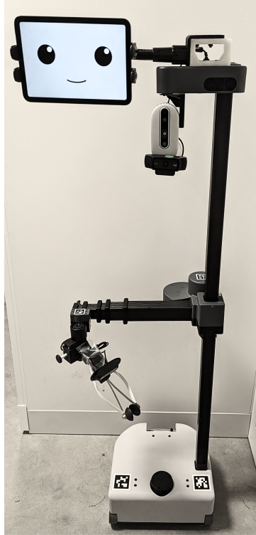
Figure 2.1. We designed an escape room study that used Stretch. It could manipulate objects in the environment and talk to people. It could perform handovers, help find objects, read encrypted data, and help with hazardous tasks.
