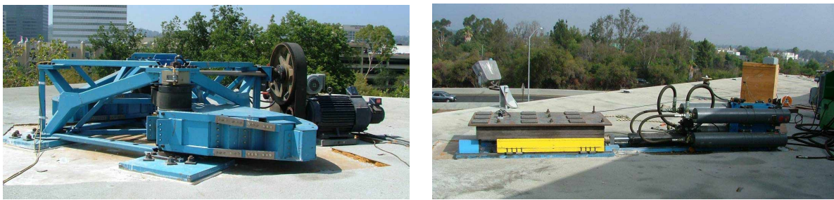
Figure 3. Field shakers, (a) Eccentric mass shaker and (b) linear shaker
