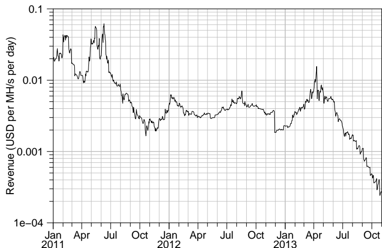
Figure 2.9. Daily miner revenue per MH/s of mining capability. Daily revenue per MH/sec of hashing power is given by 86400 \cdot D \cdot U , where D is the expected revenue in BTC per million hashes computed, and U is the USD:BTC exchange rate.
