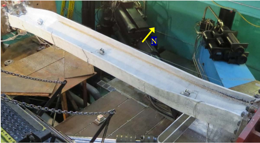
Figure 4.51 Specimen 21M-NF: Significant Twisting at East End
