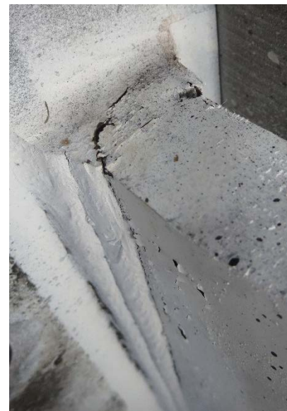
Figure 4.38 Specimen 21M-VAU: Column Flange CJP Weld Fracture
