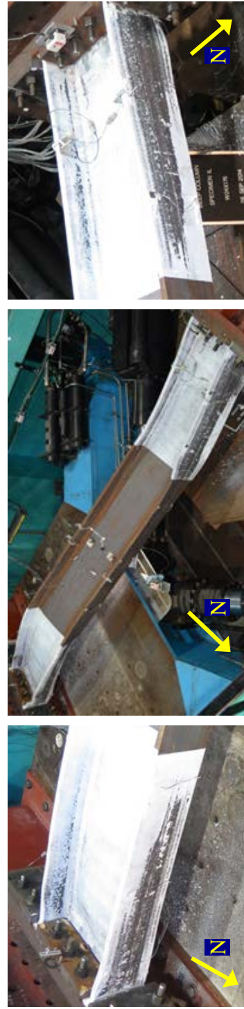
(b) Single-Curvature Coupled Buckling Mode of W18x130 Column with C_a = 0.4 (Specimen 16M)
