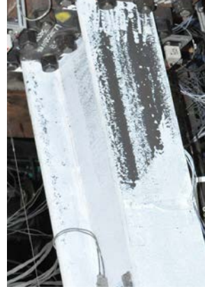
Figure 4.23 Specimen 16M: Yielding and Buckling Progression at Member Ends
