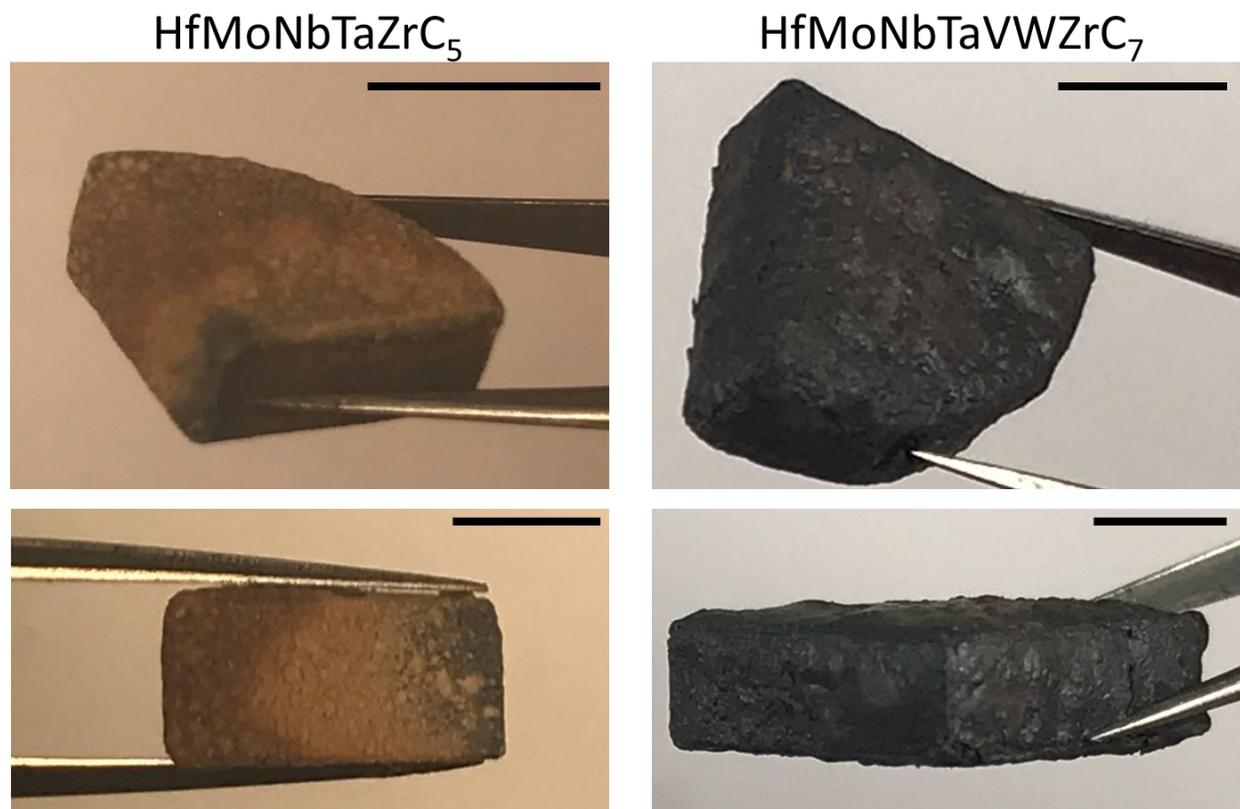
**Supplementary Figure 13 Post-oxidation images of the samples.** Macroscopic images of the two samples show differences in the oxidation behavior. The  $\text{HfMoNbTaZrC}_5$  (left) is compared with  $\text{HfMoNbTaVWZrC}_7$  (right). Scale bars 5mm.
