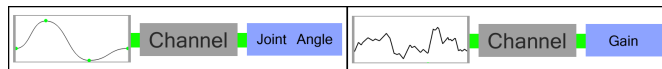
Figure 4.3: Animation nodes can be based on spline input (left) or feedback input (right).
