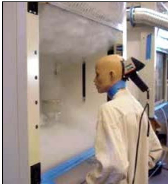
Figure 4: Prototype unit demonstrating the air divider.
