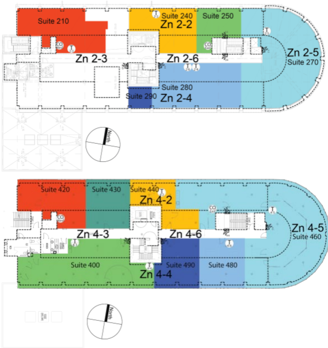
Figure B-1: Radiant zone and space layout for floors two and three in DBC. The radiant zones are outlined with black dashed lines. There is one thermostat per radiant zone. The space layouts are designated with color per floor i.e. the same color used on multiple floors does not represent the same tenant. The radiant zones are the same on floors two and four. However, the space layouts on the other two floors are different. We applied the control intervention to all radiant zone of DBC.
