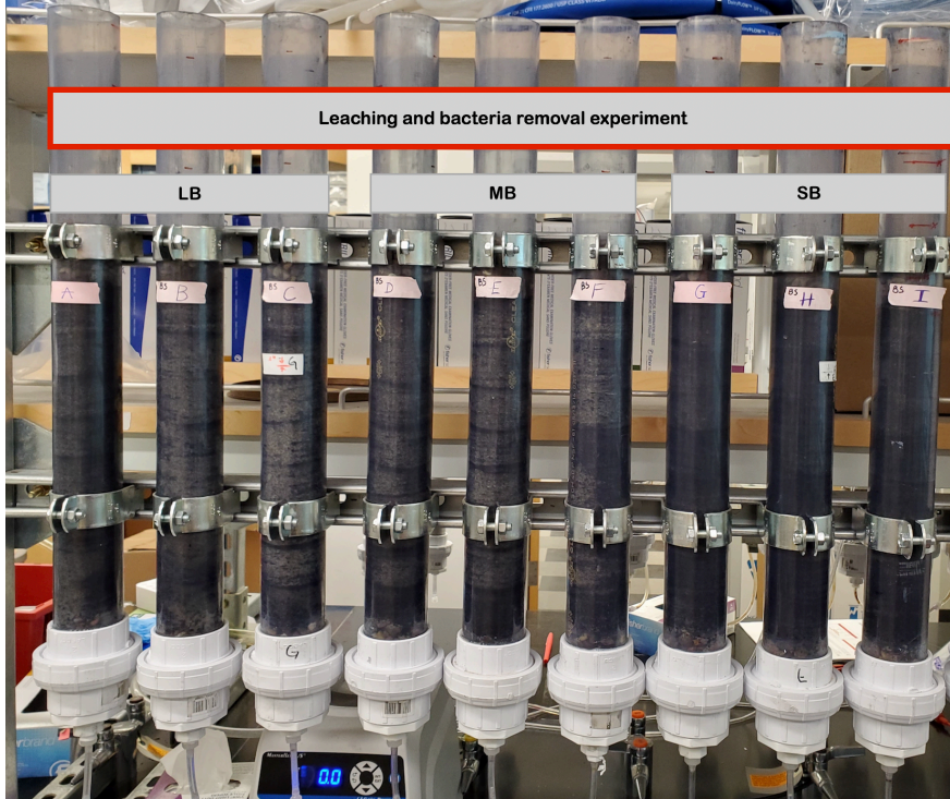
Figure 2. Triplicates columns for each biochar size fraction (total 9 columns) were used to quantify the effect of biochar particle size on their performance in biofilters subjected to compaction.
