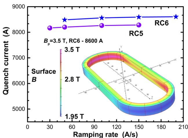
**Figure 3.** Ramp rate dependence of the quench current  $I_q$  of RC5 and RC6 during linear current ramps. Inset shows a 3D display of the contours of the surface magnetic flux density generated by RC6 at 8600 A.
