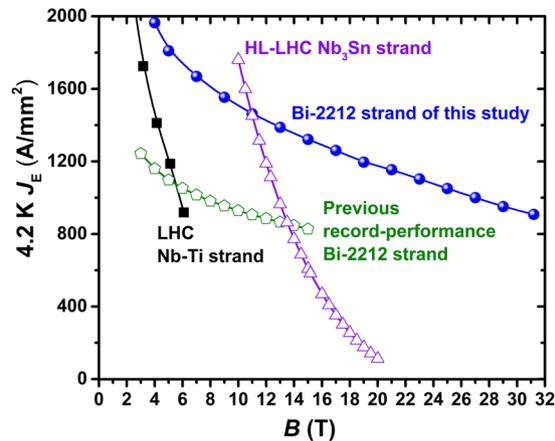
**Figure 1.**  $J_E(B)$  of an optimally processed sample of the strand used in this study in comparison to that of a Bi-2212 with the previous record performance, the LHC Nb-Ti strand, and the HL-LHC RRP Nb<sub>3</sub>Sn strand.
