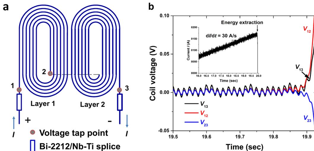
**Figure 2.** Coil voltages (RC5) during a linear current ramp (see inset in b) that ended with a quench. (a) Voltage tap map. (b) Coil voltages  $V_{13}$  (whole coil) and  $V_{12}$  and  $V_{23}$  (individual layers).
