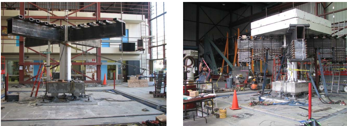
Fig. 4.2 Photographs of the pullback tests without (left) and with (right) total mass
