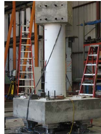
(b) Installing loadcells and the specimen on the base plate
