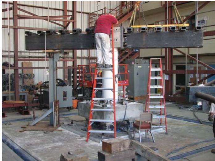
(c) Connecting the beams to the specimen by prestressing rods
