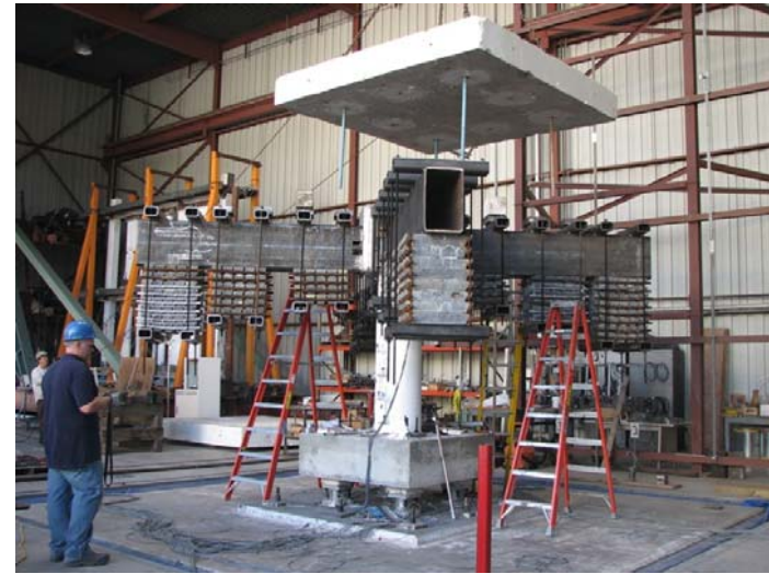
(b) Installing the first concrete block on the specimen
