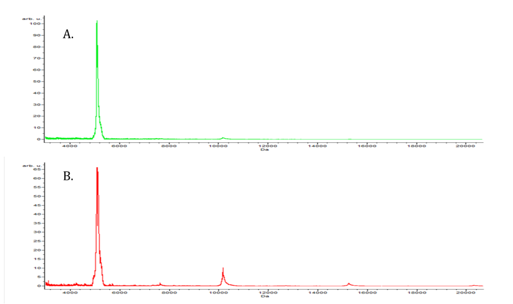
Figure 3.1: MALDI-MS spectra of Moorea producens 3L. Prepared according to literature procedure and acidified with (A.) trifluoroacetic acid and (B.) formic acid.
