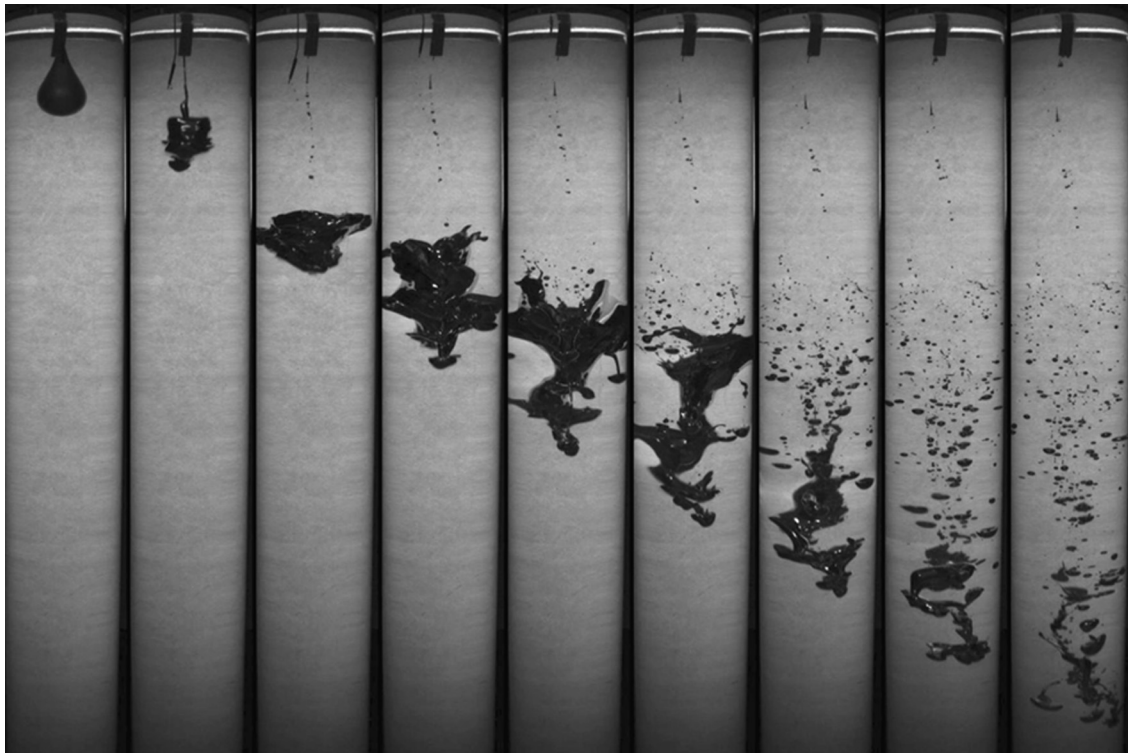
Fig. 4. Successive snapshots with a fixed time interval \Delta t = 0.18 s for a 30 mm initial radius diapir falling through pure glycerol, corresponding to Re_a = 37 , We_a = 64 and a viscosity ratio of 500. One can notice that the mean speed of the front of the diapir is rather constant.
