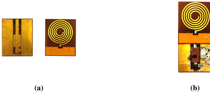
Figure 6.13. Photos of the final flexible and wireless PCB, with (a) the design of the flexible PCB on the left and the spiral antenna on the right, and (b) interfaced with the RFID IC and the sensor.
