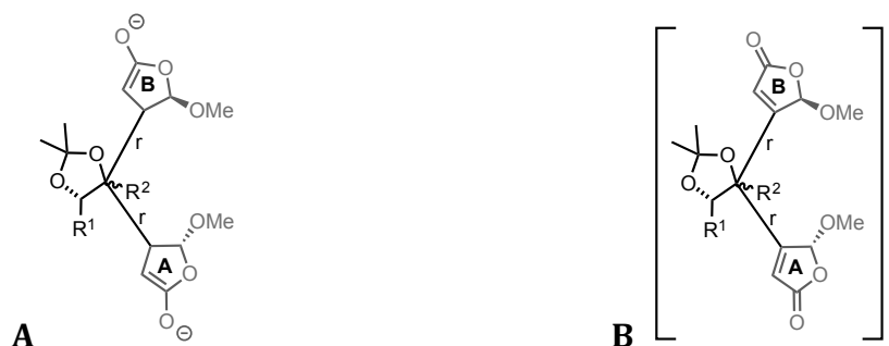
Figure S5.2. Maestro Computational Search. A. In force field calculations, the system was modified to be an enolate anion. B. In quantum chemical computations, the system was treated as radical. In both cases, the bond distance r was fixed at 2.5 Å.
