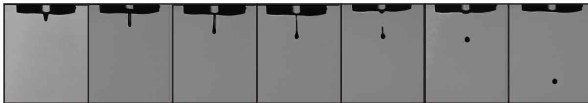
Figure S5. Droplet formation sequence for PEGDA bioink with a W_{\text{PEGDA}} of 100% and loaded with Ibuprofen at a concentration of 180 mg/mL.
