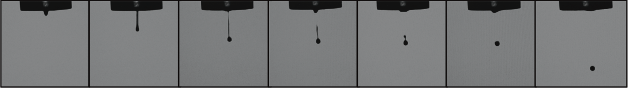
Figure 3. Bioink droplet formation picture sequence.
