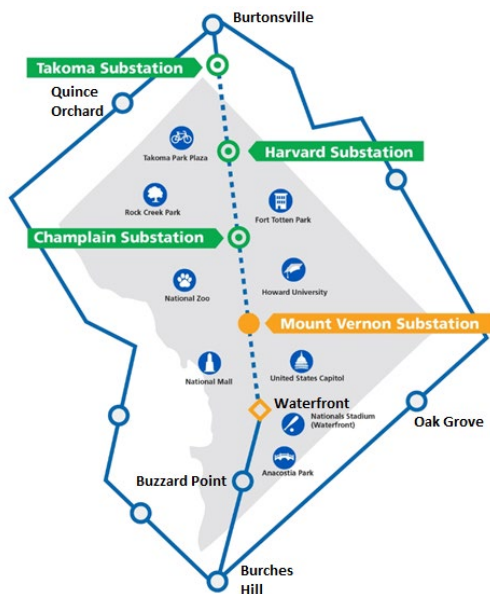
Figure 22. Pepco’s Proposed Capital Grid Project: Three Upgraded Substations (green), a New Transmission Line (dashed line), and a New Mt. Vernon Substation (Synapse 2017)
