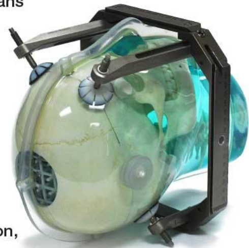
Inter-cranial Grid Phantom 335 Physical Control Points
