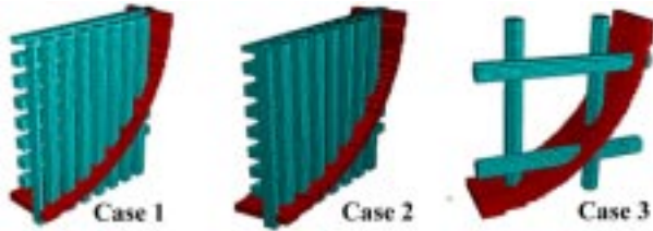
Figure 3: Gridded windows configurations modelled in MAFIA4. Left to Right: Case 1 - 15x15 grid spaced, Case 2 - 15x15 grid touching, Case 3 - 4x4 grid touching.
