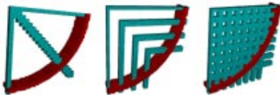
Figure 4: Other gridded windows configurations modelled in MAFIA4. Left to Right: Spider, "L" (HILAC), 15x15 grid fully overlapped.
