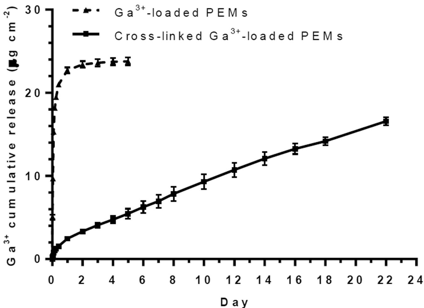
**Figure 4.** Cumulative release of Ga<sup>3+</sup> into PBS solution from either cross-linked or non-crosslinked PEMs of (PAH/PAA)<sub>60.5</sub> impregnated with a Ga<sup>3+</sup> loadings of  $24.5 \pm 0.4 \mu\text{g cm}^{-2}$ . PEMs (6 mm diameter) were incubated in PBS and the concentration of eluted Ga<sup>3+</sup> was measured by ICP-EOS. Error bars show standard deviation (n = 4).
