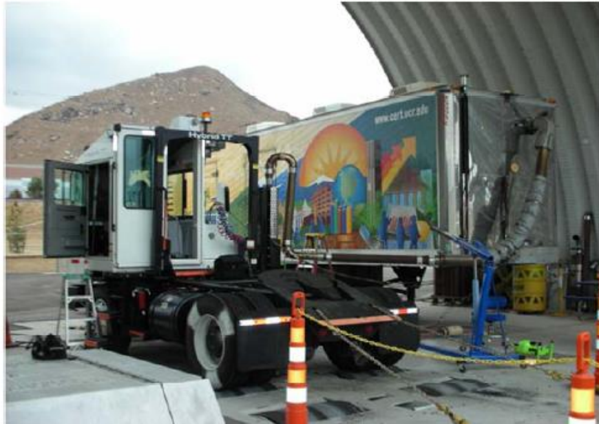
Figure D-1. UCR's heavy duty chassis eddy current transient dynamometer
