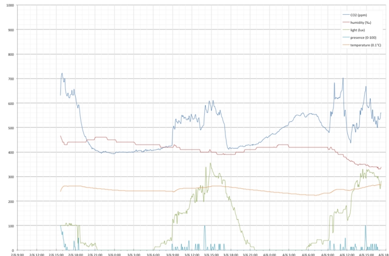
Figure 3. Objective data collected by sensor nodes placed in one of the studied offices.
