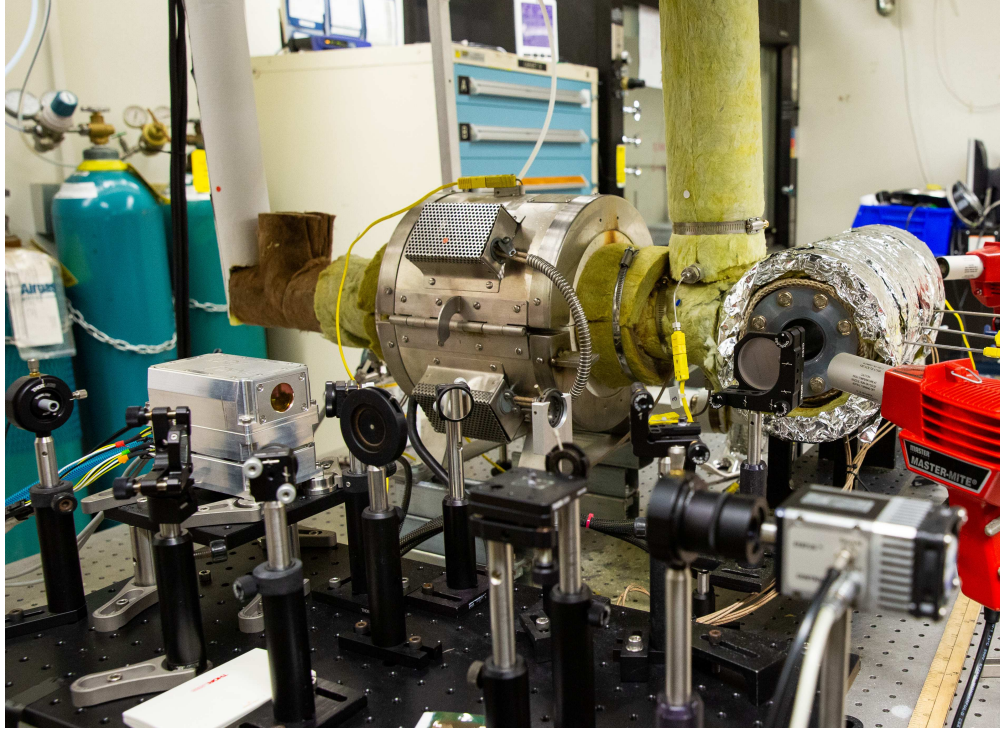
Figure 3.9: System ready to operate with OKSI ECQCL7, before the installation of water evaporator and main flow valve.
