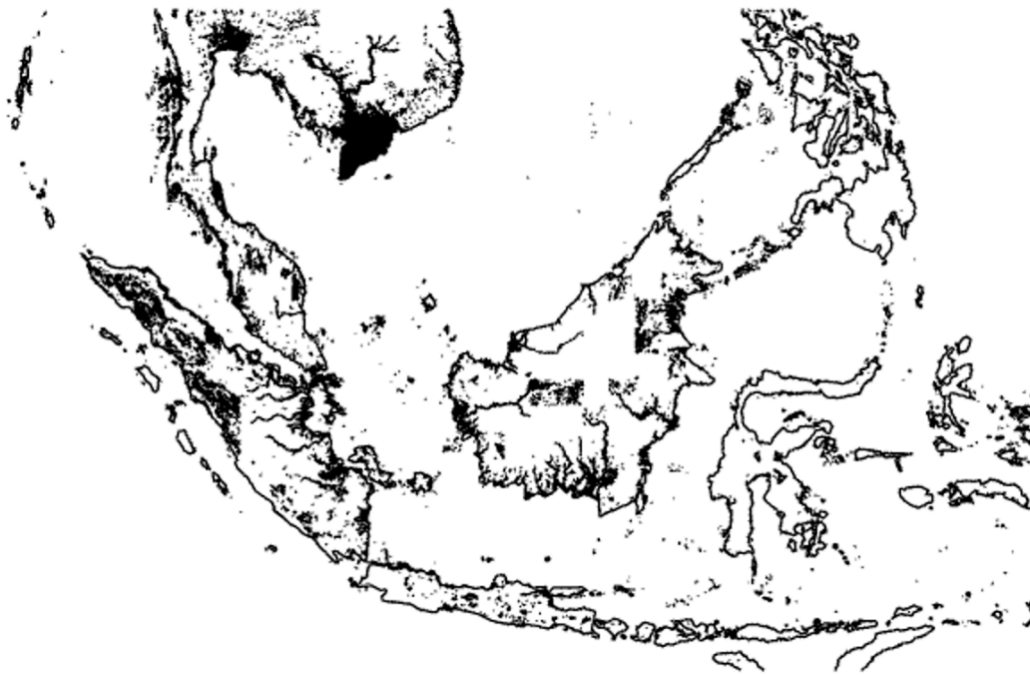
Figure 6 0m Contour lines from the Southeast Asia DEM before only seaward contours displayed.
