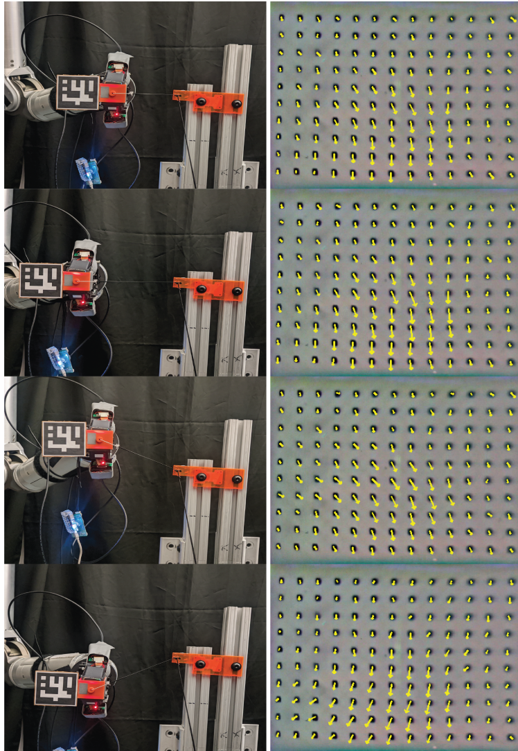
Figure 3.1: A 7-DOF robot arm controls the pose angle and tensile state of an elastic cable using a gripper outfitted with the vision-based GelSight tactile sensor [112]. One end of the tethered cable is manipulated by the gripper through a rigid rig. The left and right columns show different cable states and their tactile representations, respectively.
