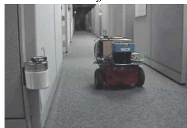
Figure 3: a) Navigation Field produced; b) Example of the path taken; c) An example of a discrete probability distribution of node k for direction (action) "East" (i.e. right); d) Experimental environment with 9 nodes; e) Path taken by the robot from node 1 to node 9; f) Mobile Robot and a Sensor Node during a real world experiment in the environment in d);
