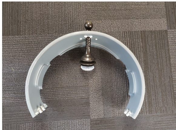
Figure 2: The top rim of a trash can is cut using a hand saw. An arch is formed by removing 160 degrees of the rim's circumference. This simulates the upper part of an ACCD.
