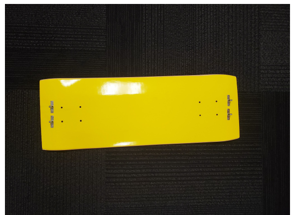
Figure 1: Two latch clips are arranged on each side of the skateboard. They are attached to the skateboard with screws. This simulates the back plate of an ACCD.
