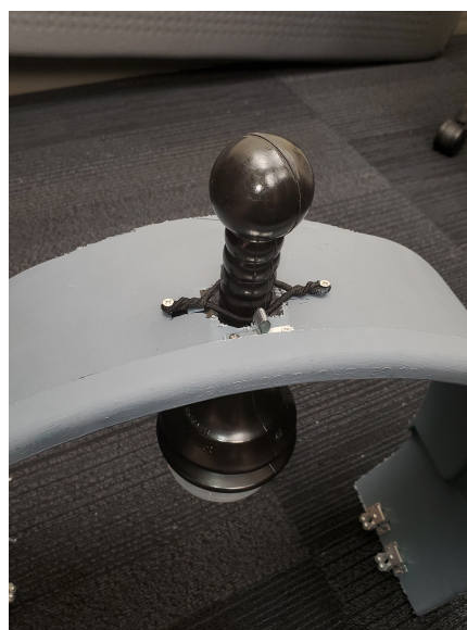
Figure 5: The plunger is suspended through a 2 inch hole on the top portion of the arch. It is held in place by a thick rubber elastic band that is wrapped around 2 screws that are on each side of the hole. There is also a latch clip glued 1 inch in front of the hole.
