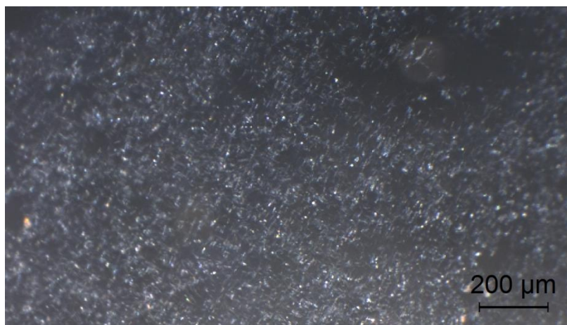
Figure 7: Photograph of a 1.25 \times 10^{-3} M Lu extraction into a 1:3 TBP:HDBP organic solution.
