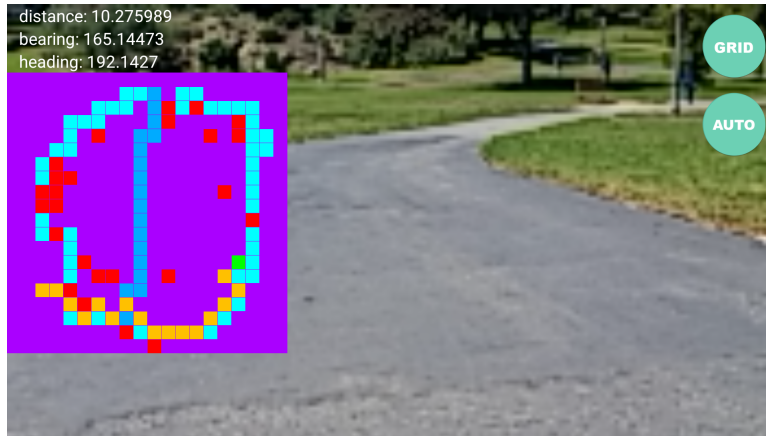
Figure 3.5: Screenshot of app used for robot navigation. The screen displays a camera view overlaid with information about distance to the destination, bearing to the destination ranging 0-360 degrees from true north, heading direction (also ranging 0-360 degrees from true north), and the 2D cost grid. Colors on the grid ranging from dark blue to red indicated the costs of the grid, with tree locations marked at highest cost in red. The planned path of the robot is indicated in yellow and the current location of the robot is marked in green. The Grid button toggles the grid view on and off and the Auto button switches the robot into and out of autonomous navigation mode.
