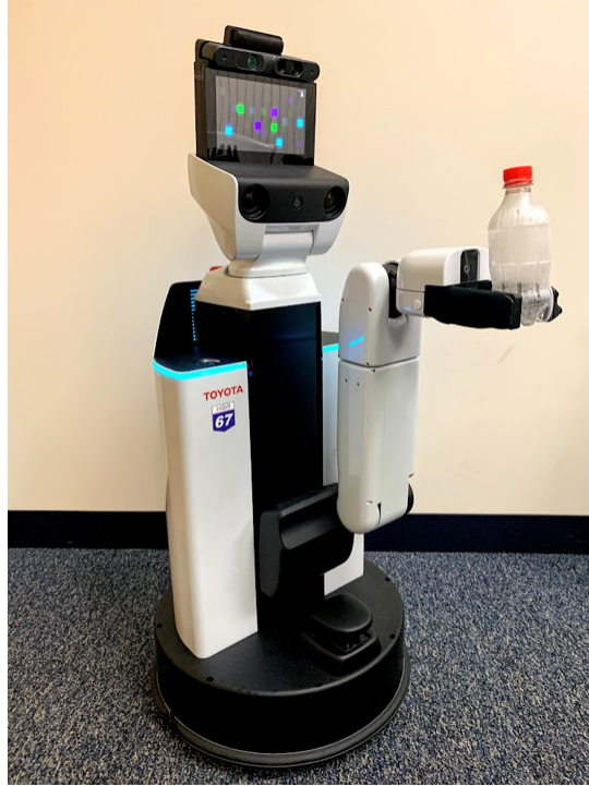
Figure 5.1: The Toyota Human Support Robot. A scanning lidar at the base allows for SLAM mapping of the environment. A combination of height, arm, and gripper controls allows for objects to be picked up and put down on various surfaces. An RGBD camera allows for object segmentation, identification, and localization.
