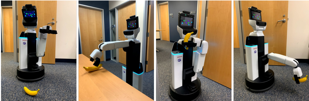
Figure 5.5: Sequence of actions in Experiment 3. The HSR was shown a banana, with nothing else in its field of view. The experimenter then placed the banana on the breakroom table, outside of the HSR's view. The robot went to the breakroom to pick up the banana and navigated to the drop off location to deposit it.
