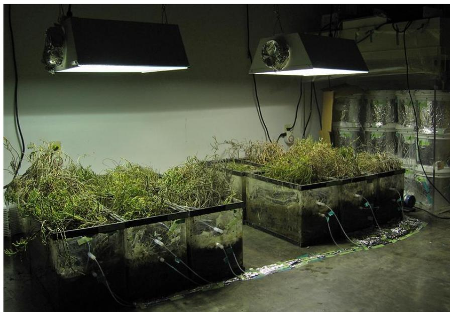
**Figure 1.** Laboratory microcosm setup including acrylic microcosms, fluoropolymer connections and lines, automated grow-lamps and peristaltic pumps, and individual microcosm reservoirs.
