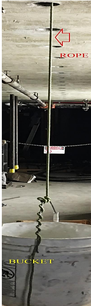
Figure (2.2): Nylon Rope Axial Test Setup
