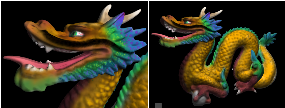
Fig. 8: Our interactive 3D paint application stores paint in a GPU-based octree-like data structure built with the Glift template library. These images show an 817k polygon model with paint stored in an octree with an effective resolution of 2048^3 (using 15 MB of GPU memory, quadlinear filtered).
