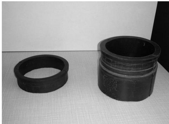
One Dura 2.0 in x 0.75 in. solid PVC reducer bushing was used inside the whole glove cuff area to hold it in place during testing (Figure 6.3). Two Dura 2.0 in. x 1.5 in. solid PVC bushings were used for glove cut outs. They were modified to create an adapter to hold a glove piece in place. Two holes were drilled in opposite ends of the bushings. Water gaskets were super-glued to the bottom of each reducer to prevent water leakage (Figure 6.4).
