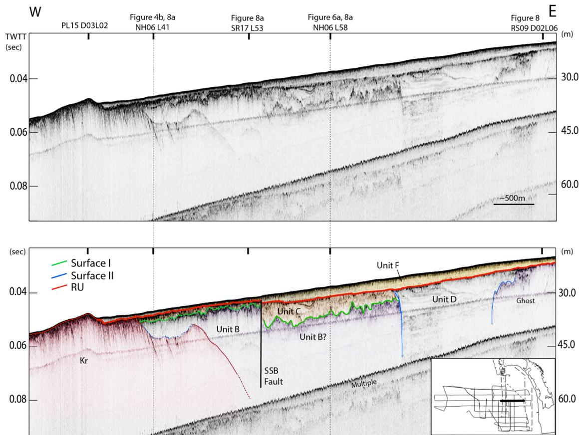
**Figure 3. Line NH06-L22, uninterpreted (top) and interpreted (bottom).** Inset shows location on map of this line (black). Perpendicular to Figure 6a, this profile shows the relationship between the Cretaceous (Kr) rock and adjacent units. The Southern Spanish Bight (SSB) Fault is observed offsetting the RU and Surface I.
