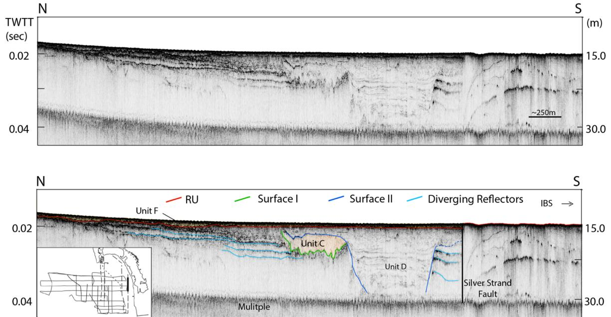
**Figure 5. Line PL15-D02L01, uninterpreted (top) and interpreted (bottom).** Inset shows location of line traced in thick black. The Regional unconformity (RU) shoals nearshore and Unit F has thinned. Profile shows offset and reflector terminations by the Silver Strand Fault (see Figure 1a). Fault offset is to the south of the channel feature and to the north of the Imperial Beach Shoal (IBS, see Figure 1).
