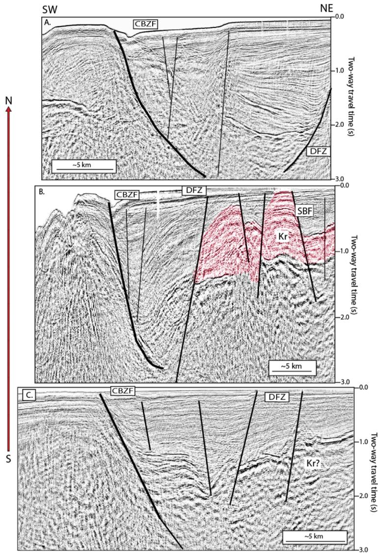
**Figure 14. Multichannel Seismic lines interpreted by Maloney (2013).** Extensional rollover on the Coronado Bank Fault Zone (CBFZ) observed to the west and normal, west dipping faulting along the western Descanso Fault Zone (DFZ). Red shading indicates interpreted location of Cretaceous geology (Kr = Rosario Group; See Figure 11 for line locations on map).
