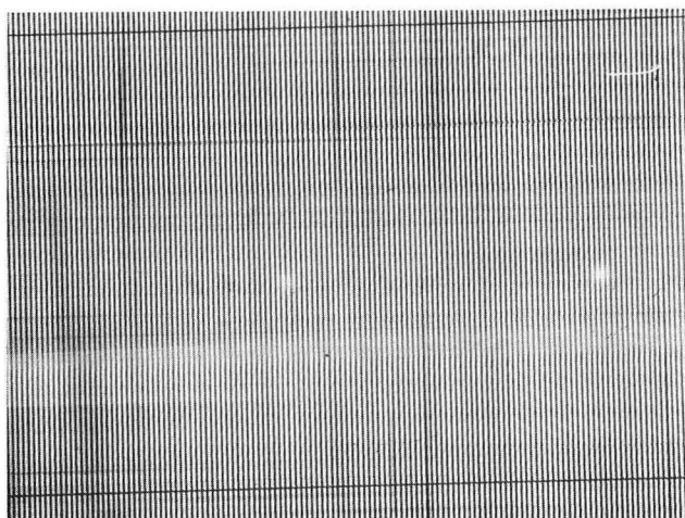
Fig. 26 Fringe pattern with a considerable difference of refractive index between the cell solution and the comparison path.
