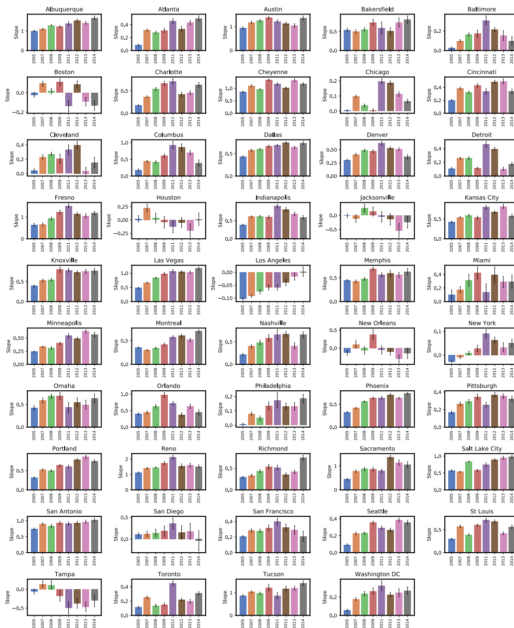
Figure C.6: The slope calculated from linear fitting between normalized OH and normalized NO 2 column among 49 cities over 8 years between 2005 and 2014, same as Fig. C.4 b) and Fig. C.5 b).
