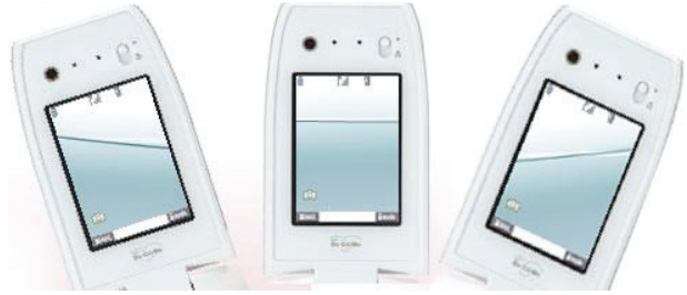
Figure 3. A mobile phone interface where battery level is indicated via the illusion of a water-filled container.
