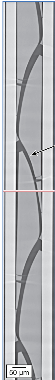
Figure 6.3: Orthogonal views and 3D rendering of pyrolysis cracks in (A) a circular microtube with 100\mu\text{m} diameter and (B) a circular microtube with 50\mu\text{m} diameter. The 3D rendering in (A) shows a section view of the crack network within the microtube. Colored lines on orthogonal views indicate intersectionality of perpendicular planes in the 3D image data.
