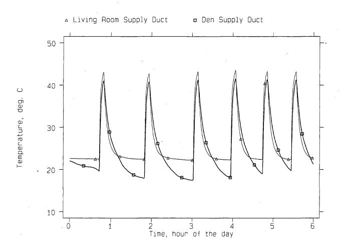
FIGURE 3. Supply-register temperature variations during normal system cycling during heating. One register decays to attic temperature during off cycle, whereas the other register decays to room temperature, suggesting a thermosiphon flow loop. Data from pilot house.
