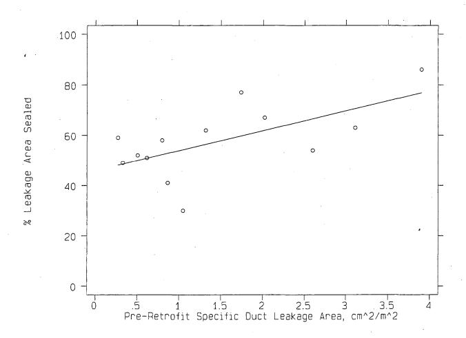
FIGURE 2. Percentage of total duct leakage sealed as a function of the duct leakage area per unit house floor area. Regression line is  $46\% + 8\% \times SLA$  ( $R^2 = 0.39$ )
