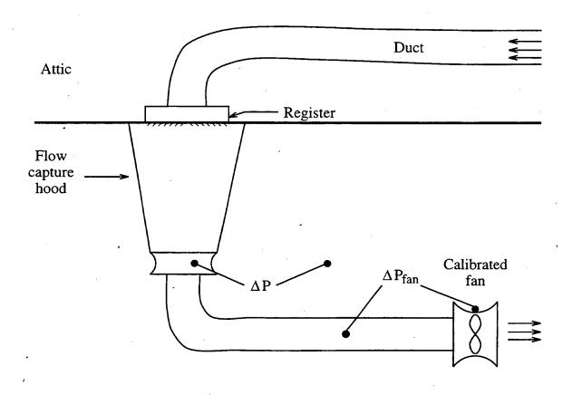
FIGURE 1. Arrangement of flow capture hood and calibrated fan demonstrating measurement of air flow out a supply register.
