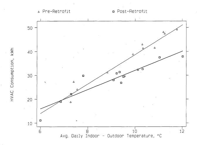
**FIGURE 4.** Daily heat-pump energy use as a function of average indoor-outdoor temperature differential before and after duct retrofit. Pre-retrofit regression line slope is 6 kWh/day  $^{\circ}$ C (R<sup>2</sup> = 0.92), and whereas post retrofit is 4 kWh/day  $^{\circ}$ C (R<sup>2</sup> = 0.86). Data for House 6.
