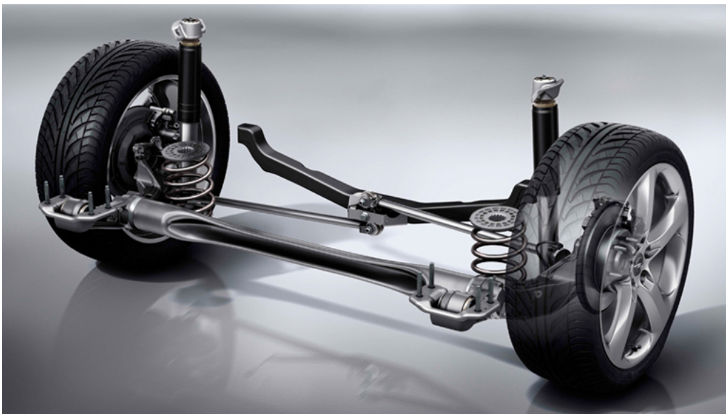
Figure 2.3: WATT'S LINKAGE USED AS THE AUTOMOBILE'S REAR WHEEL SUSPENSION 2.
