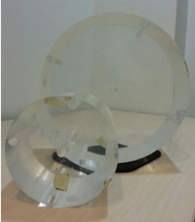
**Figure 3.5.** 16 cm head and 32 cm body CTDI phantoms.
