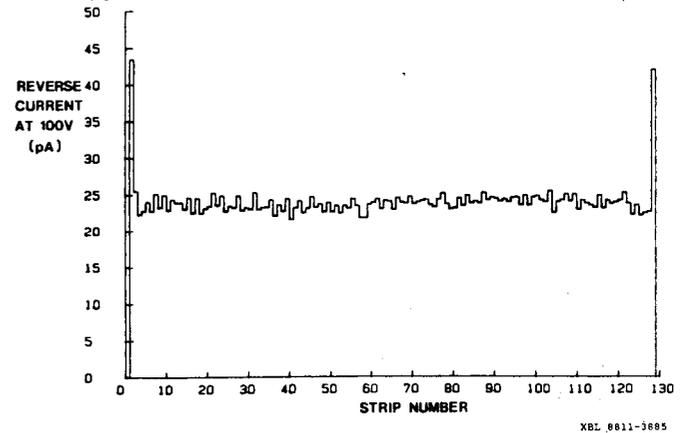
**Figure 2.** The reverse-bias current at 100V bias for the strip detector described in the text versus the strip number.
