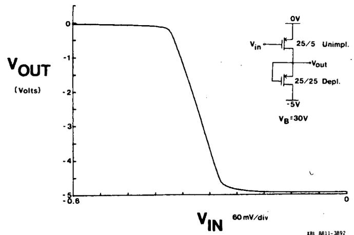
**Figure 9.** Transfer characteristics of the common-source amplifier shown in the inset. The 30V substrate bias is sufficient to overdeplete the substrate.
