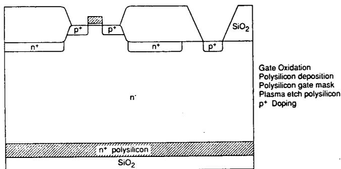
Figure 6. Device cross-section after boron doping. The device on the left is a p-channel MOS transistor while the device on the right forms a p-i-n diode.
