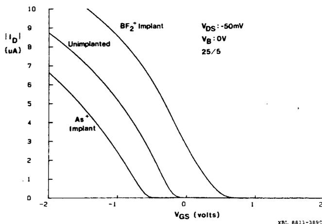
Figure 7. Linear region current-voltage characteristics for p-channel devices fabricated on high-resistivity silicon.
