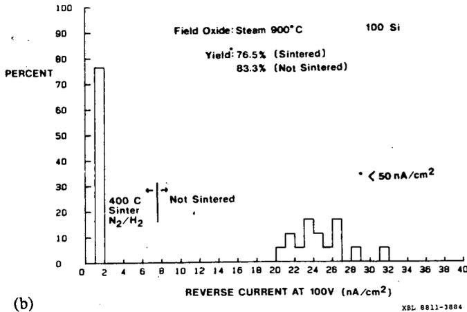
**Figure 1.** The distribution of reverse-bias leakage currents for 2 mm diameter diodes before and after sintering in forming gas at 400C for 20 minutes. The detector bias voltage was 100V.
