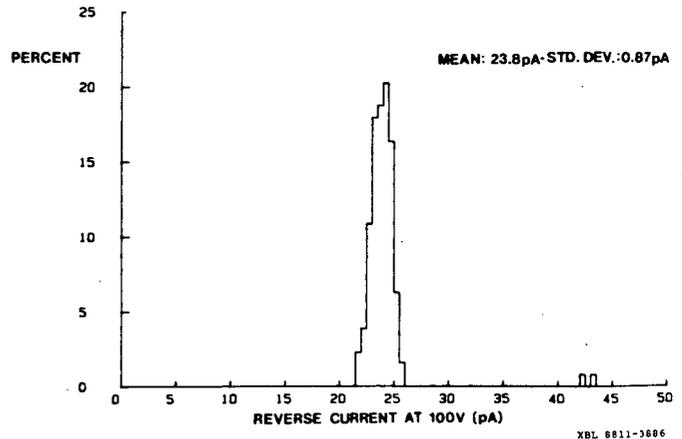
**Figure 3.** The distribution of reverse-bias currents for the strip detector from Figure 2. The statistics do not include the edge strips.
