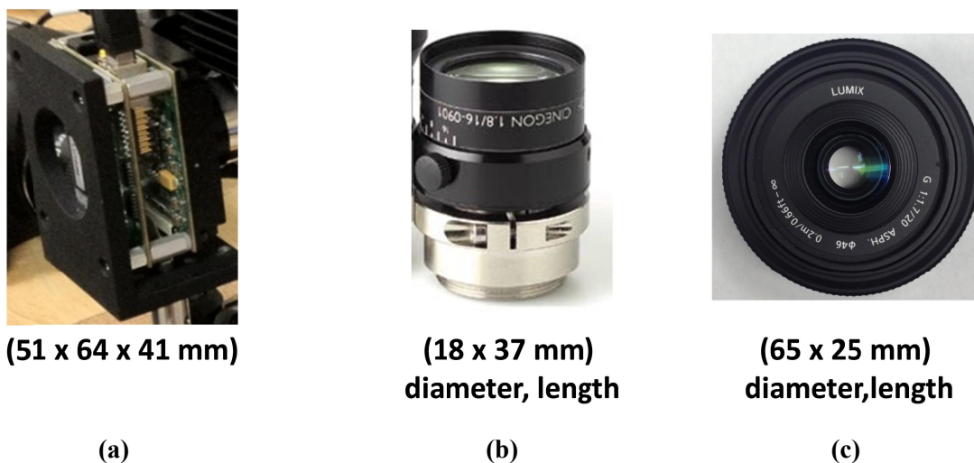
Figure 4 – Camera components tested in this study, including a CCD detector (a), and a research (b) and COTS (c) grade lens
